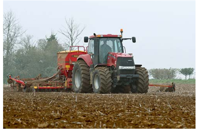
Once finished on the subsoiler the Case IH Magnum 310 moves on to drilling NDR's winter wheat area with a 6m Väderstad Rapid drill.
